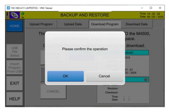
The DOWNLOAD process will restore (write) the PLC program (previously backed up to the HMI). This process should complete in about 90 seconds.
