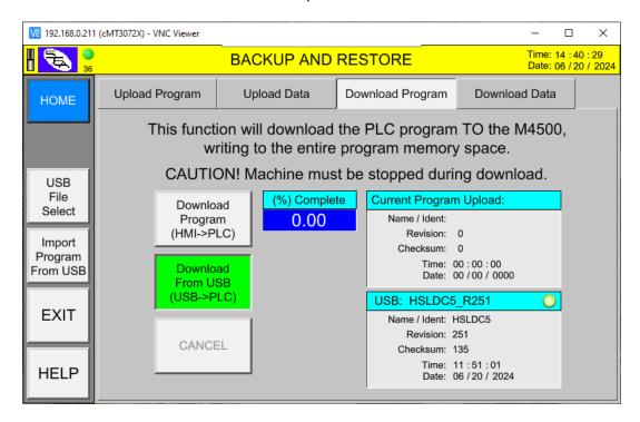
Select the "Download Program (HMI->PLC)" button. This will initiate the download process using the information from the selected "expanded memory" file (.emi) of the USB thumb drive.
