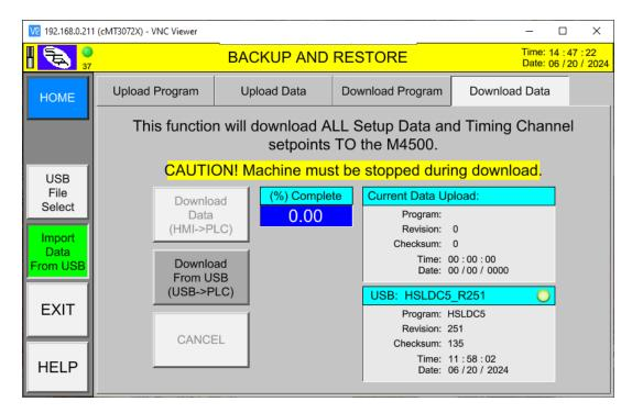
A popup will be displayed confirming the choice of operation. Select "OK" to initiate and continue with the "Import" operation or "Cancel" to abort. This operation will import (copy) the setup data (and timing channel setpoints) to the HMI, overwriting the previously saved setup data.
