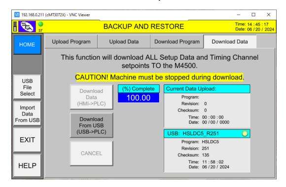
Although the PLC program and setup data have been restored, this information can also be imported into the HMI from the selected USB expanded memory file (.emi).
