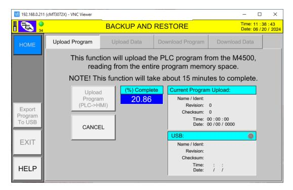
Once the upload is at 100% Complete, the **Current Program Upload** will show the Name, Revision and Checksum of the current program uploaded, as well as a time and date stamp of when it was completed.
