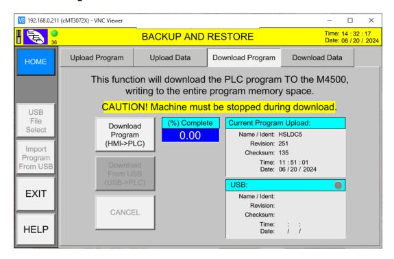
Select the "**Download Program (HMI→PLC)**" button to initiate the DOWNLOAD process of writing the PLC program to the M4500. This process should complete in about 90 seconds.
