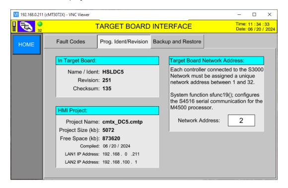
Select the "Backup and Restore" TAB and then select "Upload Program (PLC->HMI)" button:
