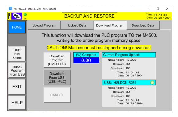
The import function is generally a two step process. After importing the PLC program, the previously saved setup data can also be imported (but isn't required). From the Download Data TAB, select the "Import Data from USB" button.
