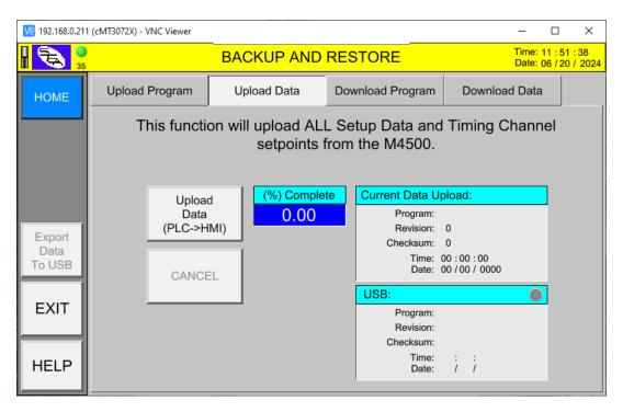
Selecting the "**Upload Data (PLC->HMI)**" button will initiate the UPLOAD process of reading the setup parameters and timing channel setpoints from the M4500.
