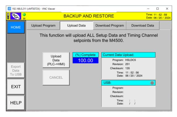
**Exporting TO an "expanded memory" file (.emi) on a USB thumb drive**: Once the PLC program and setup data have been uploaded to the HMI, the data can optionally be **exported TO** an "expanded memory" file (.emi). To perform this function, insert a USB thumb drive into the USB port (located next to the RS-232 serial communications port) on the back of the HMI.
