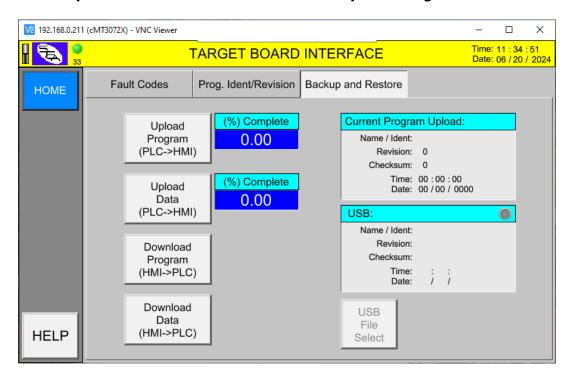
This will initialize to the "Upload Program" TAB. Select the "**Upload Program (PLC->HMI)**" button to initiate the UPLOAD process of reading the PLC program memory space from the M4500.
