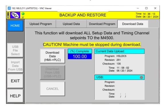
Alternatively, the PLC program and seup parameters can be **downloaded FROM an "expanded memory" file (.emi) on a USB thumb drive**. With the USB thumb drive inserted into the USB port of the HMI the "USB File Select" button will become active (button is gray when NOT active).
