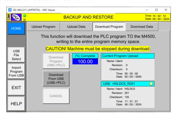
From the Download Data TAB, select the "**Download from USB (USB->PLC)**" option and then select the "**Download Data (HMI->PLC)**" button.
