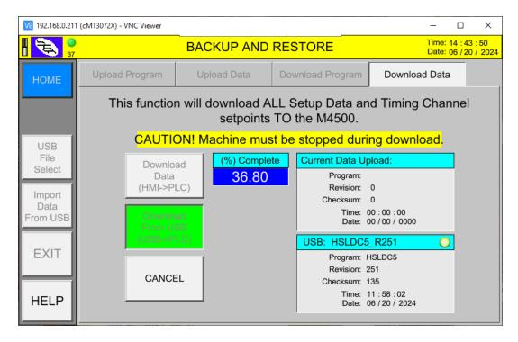
Note: The "CANCEL" button is used to TERMINATE the process at anytime.
