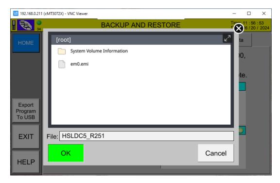
Once the export process is complete, the header for the "USB:" information will display the name of the selected ".emi" file, as well as the information in the data area below will match that of the "Current Program Upload".
