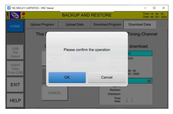
The DOWNLOAD process will restore (write) the setup parameters and timing channel setpoints to the M4500 (previously backed up to the HMI). This process should complete in about 90 seconds.
